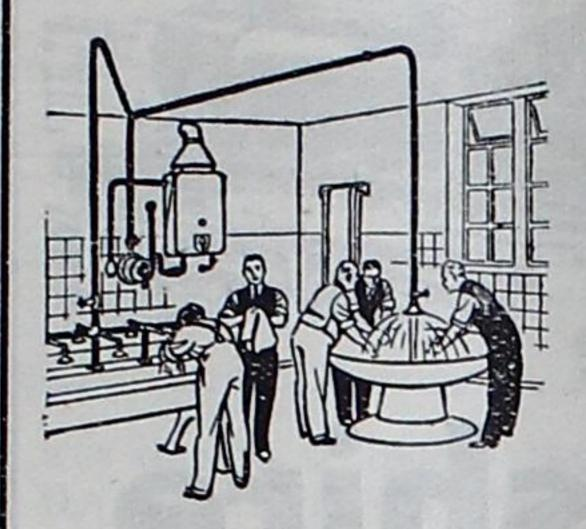
Wherever there is group washing there is waste unless Leonard-Thermostatic Water Mixing Valves are fitted. With a Leonard-Thermostatic Valve you can fix the temperature of the hot water at the most suitable point and lock it. The valve will keep the temperature steady no matter how the pressures fluctuate in the supplies. Leonard-Thermostatic
