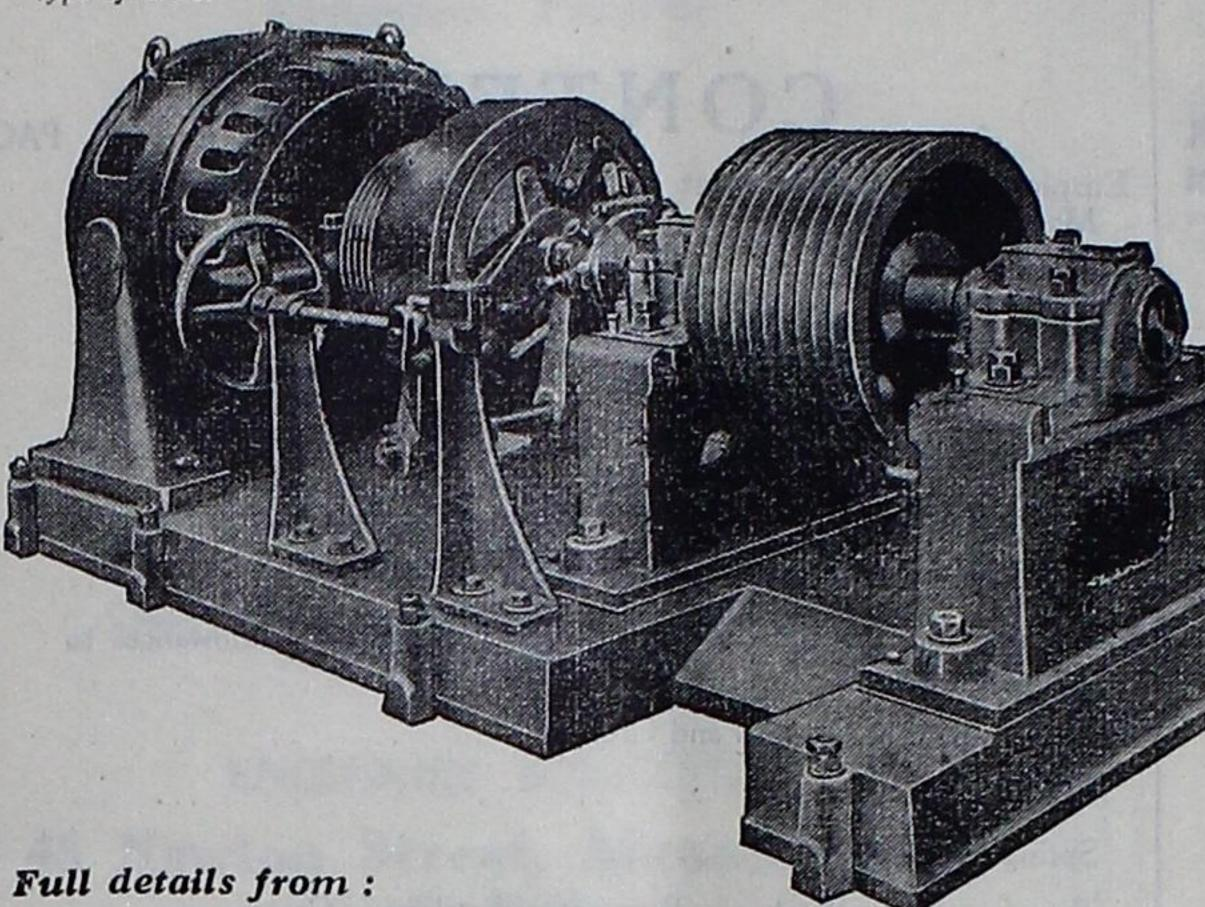
From a standpoint of pure expediency there is everything to be gained by fitting thoroughly dependable guards and clutches. The smooth, speedy manner in which a Heywood & Bridge clutch picks up and releases its load greatly reduces the wear on gearing and drives whilst giving a maximum margin of safety; whilst calenders and all machines involving rolls can be operated with much greater efficiency when the operative knows he is completely protected by efficient nipguards.
