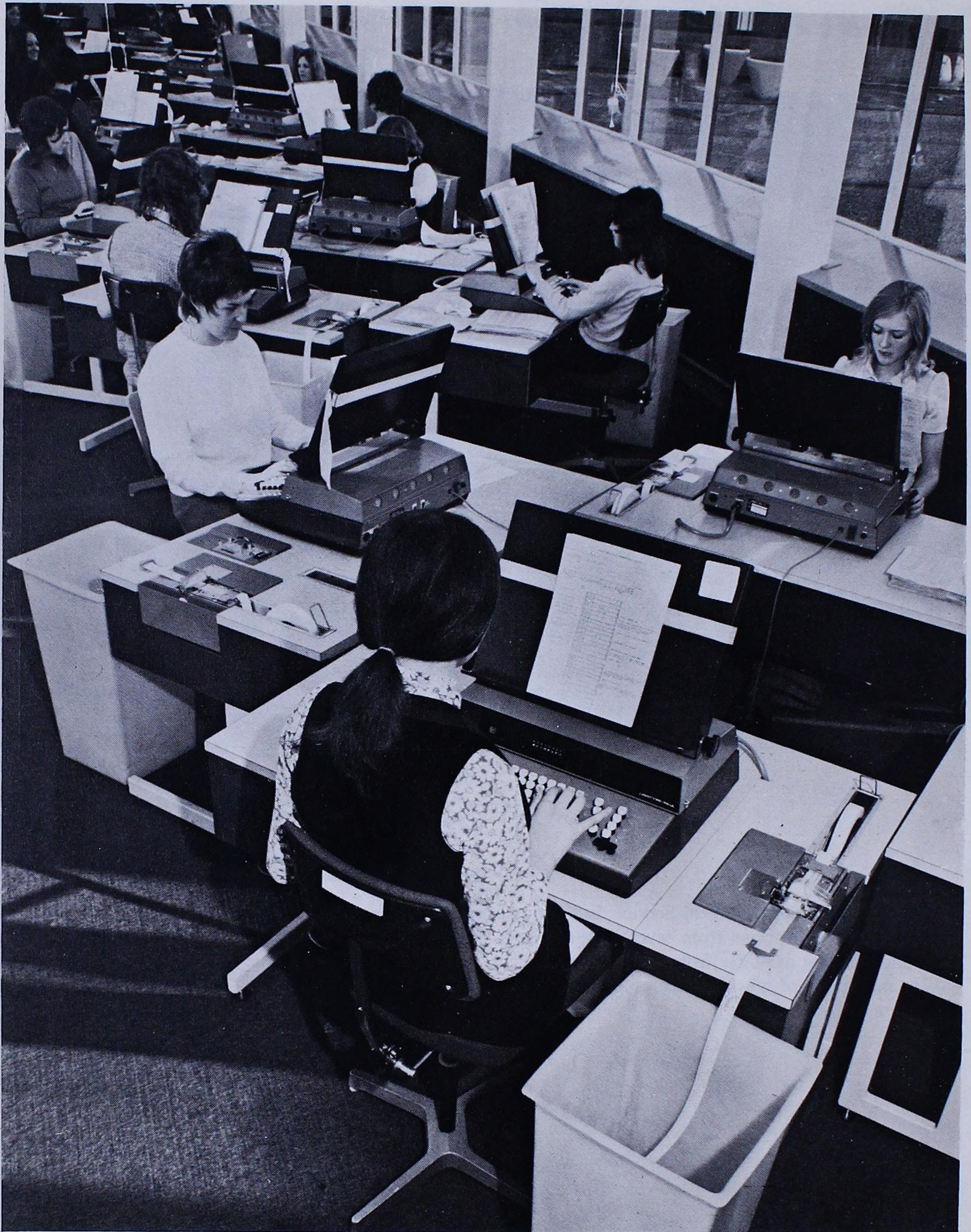
Operators preparing punched paper tape for the 1906 computer complex at the new Business Statistics Office building in Newport.
